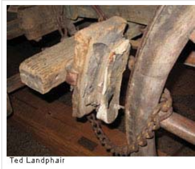
That's an ordinary shoe, all right, between the pieces of wood in the braking device of an old Conestoga wagon
